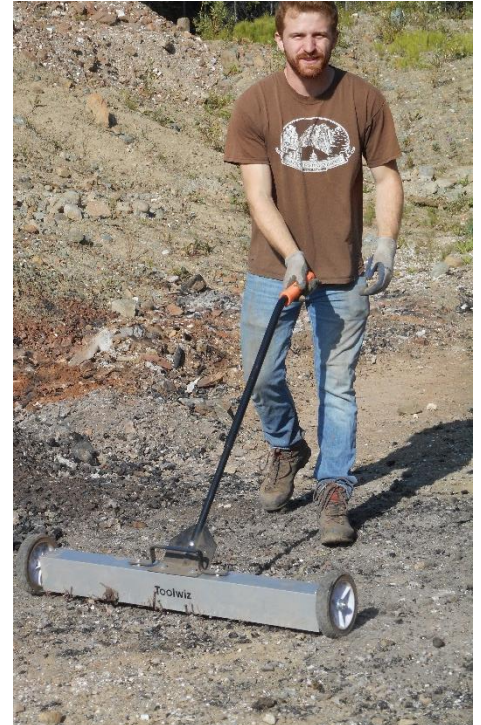
Figure 12. CGC employee using a magnetic tool to remove any traces of scrap metal, such as nails or screws from a reclaimed site
