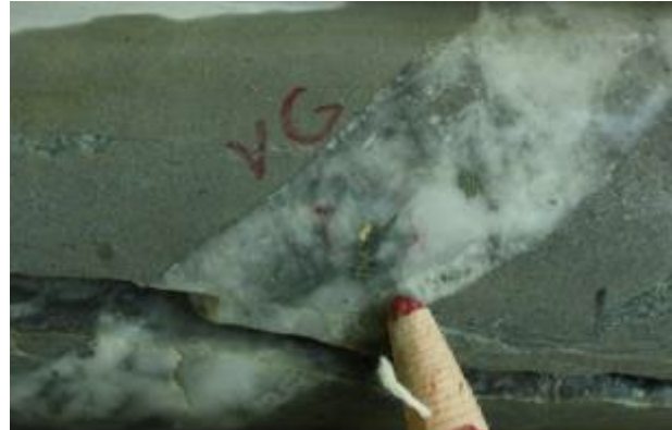
Free gold in extension vein (T4), drill hole TA09-25
