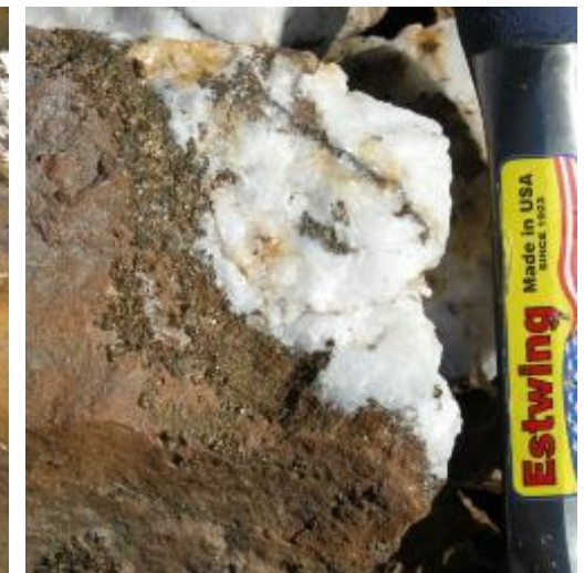
Vein with T3 coarse pyrite envelope
