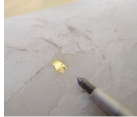
Free gold in extension veins, drill hole TA09-41
