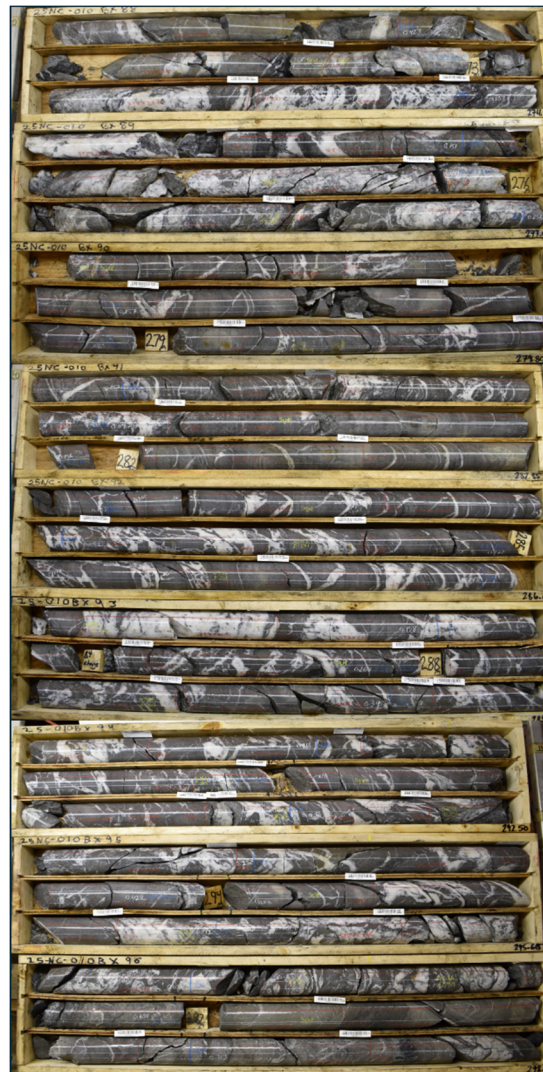
Figure 6. Drill core photos from drill hole 25NC-010 showing a broad intercept of high density narrow sheeted veining hosted in sulphide-mineralized and altered mafic volcanic host rock. Assay results remain pending.
