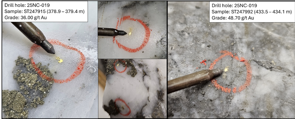
Figure 17. Visible gold in drill hole 25NC-019 observed in quartz veins hosted in Fe-carbonate-sericite altered and sulphide-mineralized basalt.
