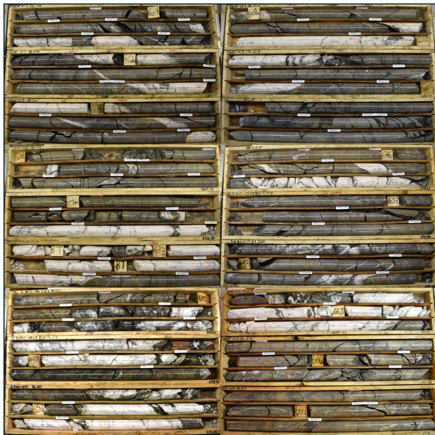
Figure 7. Drill core photos from drill hole 25NC-013 showing a broad intercept of high-density sheeted quartz veining hosted in variably sulphide-mineralized and altered mafic volcanic host rock. Assay results remain pending.
