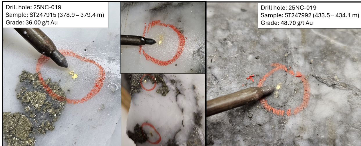
Figure 10. Visible gold in drill hole 25NC-019 observed in quartz veins hosted in Fe-carbonate-sericite altered and sulphide-mineralized basalt.
