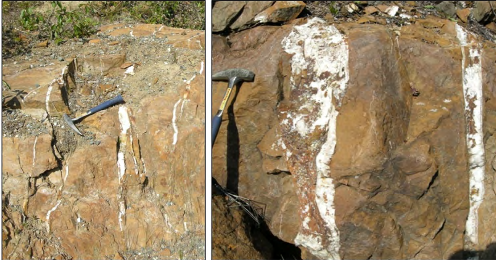
Examples of east-west trending sheeted vein sets with gold-bearing iron carbonate and sericite alteration envelopes observed in outcrop from the Newcastle target area at Cassiar North.
